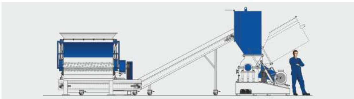
System example for a Two-Stage Recycling Plant with a ZSS 1500, one conveyor feed belt and a GSH Granulator
