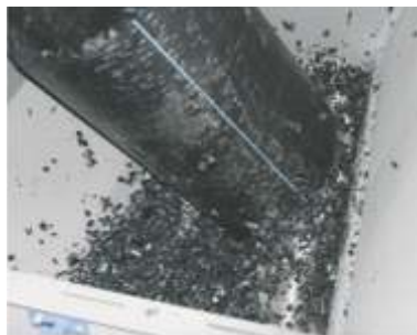
Pipe application, pre-grinding of pipes, for continued processing in a granulator.
